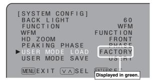
**3** When the file whose data is to be loaded is selected from the FACTORY or USER1 to USER5 files and the FUNCTION/ENTER button is then pressed, the screen shown below appears.
